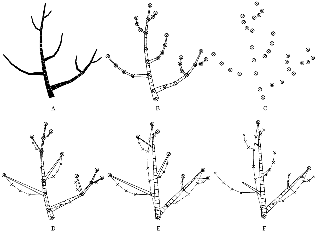
FIG. 3. Approximation strategies for digitizing a monopodial branching system. A, A monopodial branching system. Two axes have been decomposed into sub-components (e.g. internode units). B and C, Precise modelling of the branching system geometry would require recording all the 3D points (denoted by \otimes ). D, Digitized points not corresponding to branching points have not been recorded ( \times ). E, Only the extremities of the branching system axes have been recorded. F, Only the extremities of the two major axes have been recorded.
